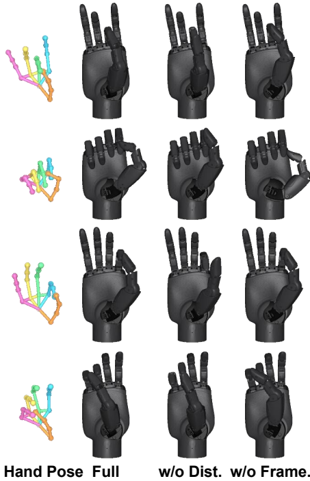
Figure 11: Retargeting ablation. The distance objective maintains pinch closure, and the frame objective preserves thumb opposition.
